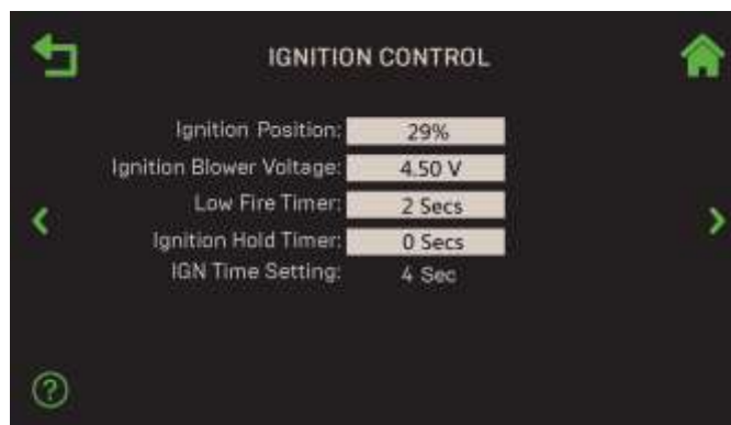
Figure 6-81 : Fire Control : Ignition Control
