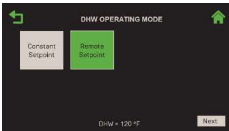
Figure 2-74 : BST Manager – DHW & Other : DHW Operating Mode
