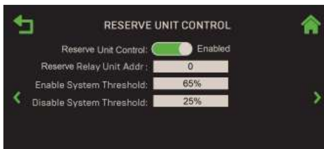
Figure 6-44 : Écran Operating Controls : Reserve Unit Control
