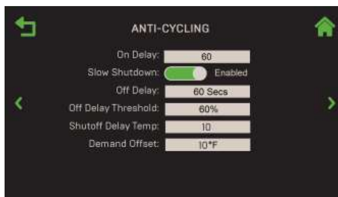
Figure 6-41 : Écran Operating Controls : Anti-Cycling Control
