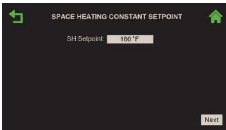
Figure 2-44 : Écran BST Manager – Space Heating : Constant Setpoint
