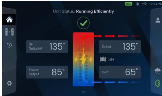
Figure 4-4: Unit Dashboard Screen – Running Efficiently
